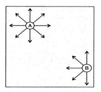
The force on the single molecule at the surface will obliviously proportional to the number  $n_v$  of the attracting molecule per unit volume.
