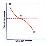
Hence at critical point C, we have  $\frac{\partial p}{\partial V} = 0$  and  $\frac{\partial^2 p}{\partial V^2} = 0$ .
