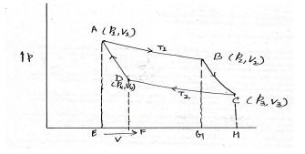
Fig : 2 Indicator Diagram
