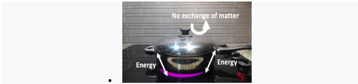
Figure 2. This is a closed system. The system is the pan/lid and the surrounding is the kitchen.
